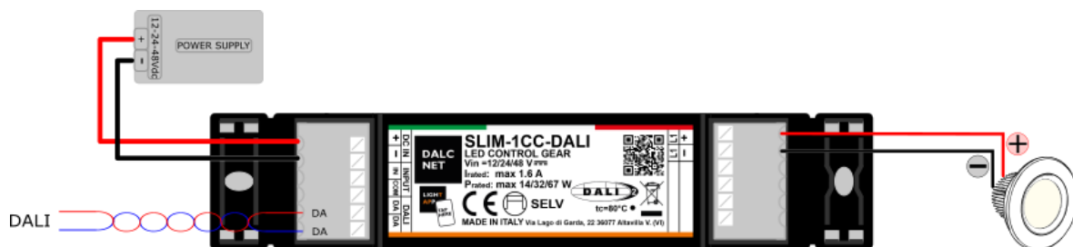
Figure 2: Connection diagram for White or Single-Colour LED loads
